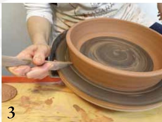
3 Angle the ring slightly outward. Create a bevel with a wooden knife as a cut-off guide.
